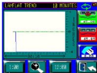
LF-Sizer Layflat trends can be viewed in 10 min., 1 hour and 12 hour periods with a zoom feature
